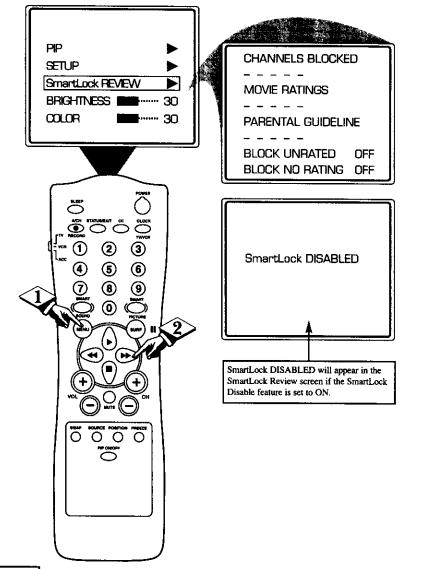
CHANNELS BLOCKED - Shows all blocked channels that where set within the CHANNELS BLOCKED feature. Up to 5 channels may be blocked at one time.
